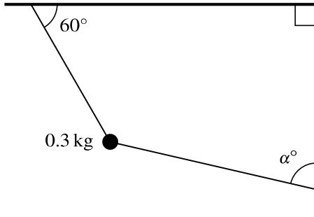
A particle of mass 0.3 kg is held at rest by two light inextensible strings. One string is attached at an angle of  $60^\circ$  to a horizontal ceiling. The other string is attached at an angle  $\alpha^\circ$  to a vertical wall (see diagram). The tension in the string attached to the ceiling is 4 N.
