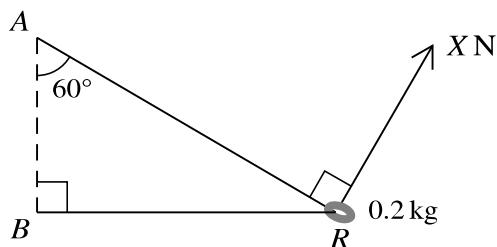
A smooth ring  $R$  of mass  $0.2\text{ kg}$  is threaded on a light string  $ARB$ . The ends of the string are attached to fixed points  $A$  and  $B$  with  $A$  vertically above  $B$ . The string is taut and angle  $ABR = 90^\circ$ . The angle between the part  $AR$  of the string and the vertical is  $60^\circ$ . The ring is held in equilibrium by a force of magnitude  $X\text{ N}$ , acting on the ring in a direction perpendicular to  $AR$  (see diagram).
