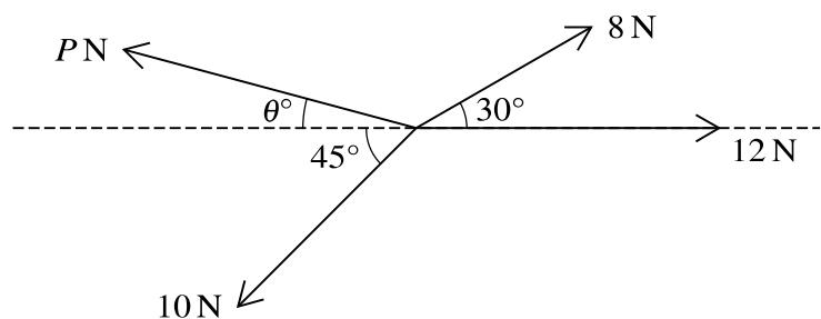
Coplanar forces of magnitudes 8 N, 12 N, 10 N and  $P$  N act at a point in the directions shown in the diagram. The system is in equilibrium.
