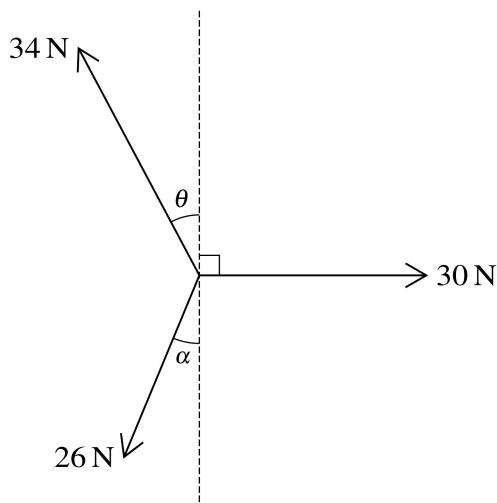
Coplanar forces of magnitudes 34 N, 30 N and 26 N act at a point in the directions shown in the diagram.
