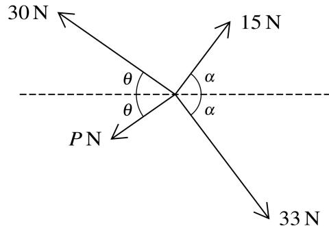
Coplanar forces of magnitudes 30 N, 15 N, 33 N and  $P$  N act at a point in the directions shown in the diagram, where  $\tan \alpha = \frac{4}{3}$ . The system is in equilibrium.
