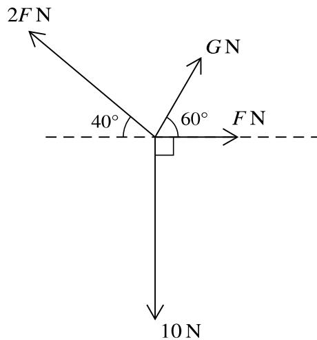
Four coplanar forces act at a point. The magnitudes of the forces are  $10\text{N}$ ,  $F\text{N}$ ,  $GN$  and  $2F\text{N}$ . The directions of the forces are as shown in the diagram.
