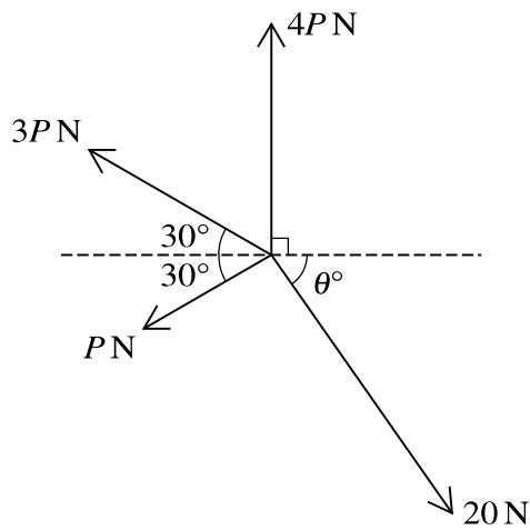
Coplanar forces of magnitudes  $20\text{ N}$ ,  $P\text{ N}$ ,  $3P\text{ N}$  and  $4P\text{ N}$  act at a point in the directions shown in the diagram. The system is in equilibrium.
