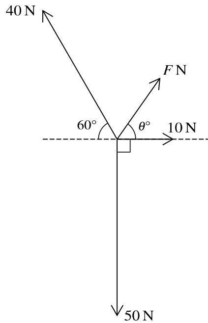
Four coplanar forces act at a point. The magnitudes of the forces are  $FN$ , 10N, 50N and 40N. The directions of the forces are as shown in the diagram.
