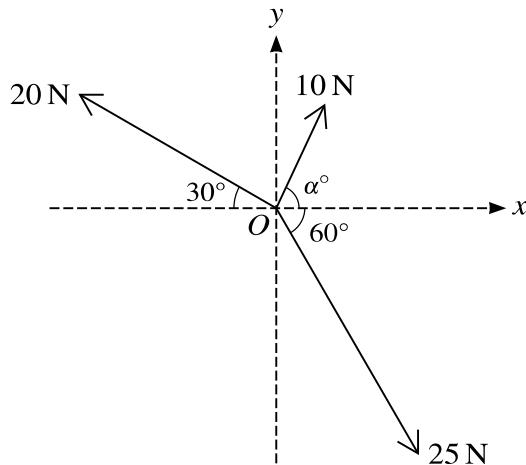
Three coplanar forces of magnitudes 10 N, 25 N and 20 N act at a point  $O$  in the directions shown in the diagram.
