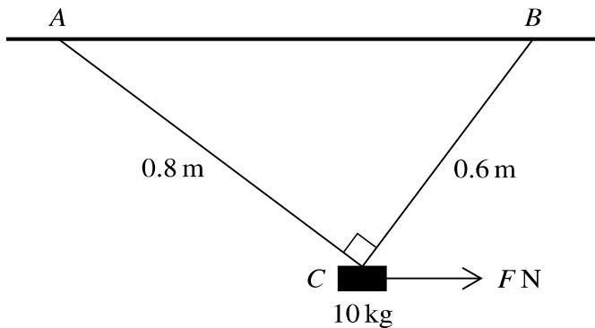
The diagram shows a block of mass 10 kg suspended below a horizontal ceiling by two strings  $AC$  and  $BC$ , of lengths 0.8 m and 0.6 m respectively, attached to fixed points on the ceiling. Angle  $ACB = 90^\circ$ . There is a horizontal force of magnitude  $FN$  acting on the block. The block is in equilibrium.
